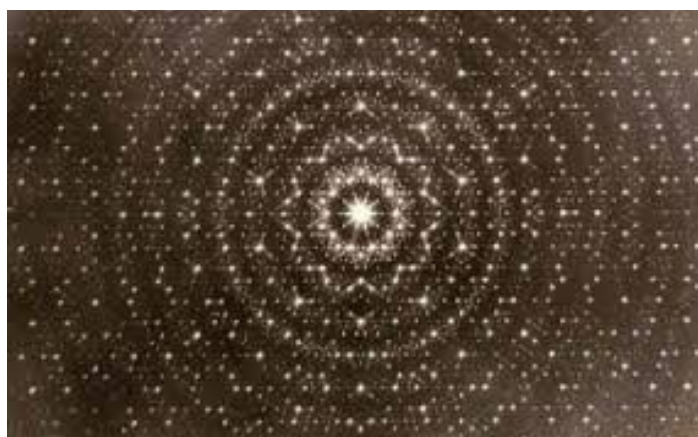
Fig. 19: Mackay's simulated diffraction pattern from a Penrose tiling
