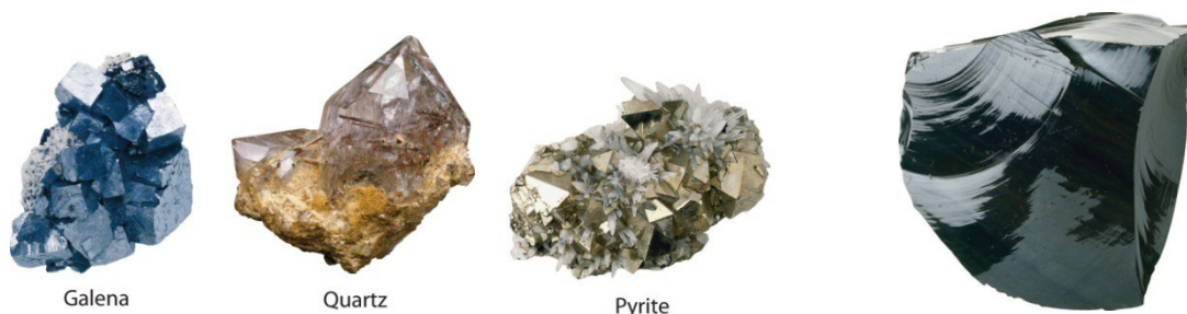
Fig. 3: Crystalline faces: the faces of crystals can intersect at right angles, as in galena (PbS) and pyrite (FeS 2 ), or at other angles, as in quartz. (Courtesy U C Davis, ChemWiki)
